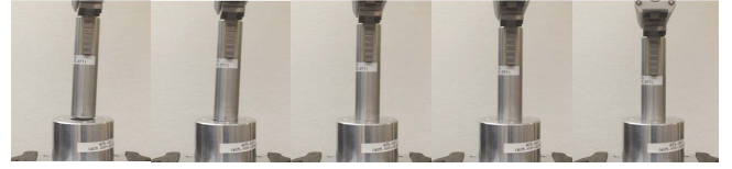
Fig. 11. Process of Robot Autonomous Insertion with Initial Orientation Misalignment.
